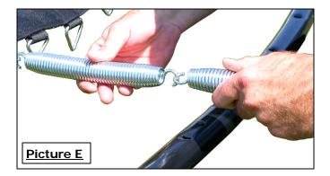
**Note:** If you are having a hard time pulling each spring toward you and hooking it into the notches on the frame, use a second spring to hook onto the one you are pulling (see Picture E, left). This will give you more leverage and make pulling the springs to the notches much easier.
