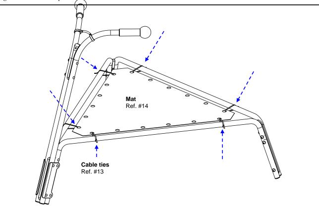
**4)** Position mat face up on ground, in center of trampoline. Top of mat edge will be smooth, and bottom edge will have a layer of material sewn to it. Temporarily secure the jumping mat to the frame with 6 cable ties (2 in each corner), as shown. **Make sure mat is pulled tight, and centered.**
