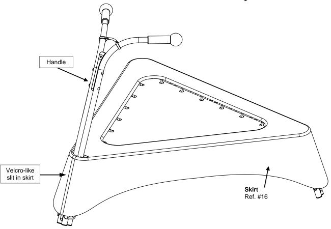
7) Open Velcro-like slit in skirt. Then wrap skirt around frame and close slit around the handle to secure the skirt in place.
