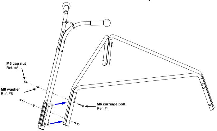
**3)** Secure handle assembly to frame, first positioning the assembly in place, then installing the 2 bolts as shown. **The handle assembly installs on the frame corner where you installed only the top bolt from Step 1.** *M6 bolts should only be hand-tight.* They will be securely tightened in a later step.
