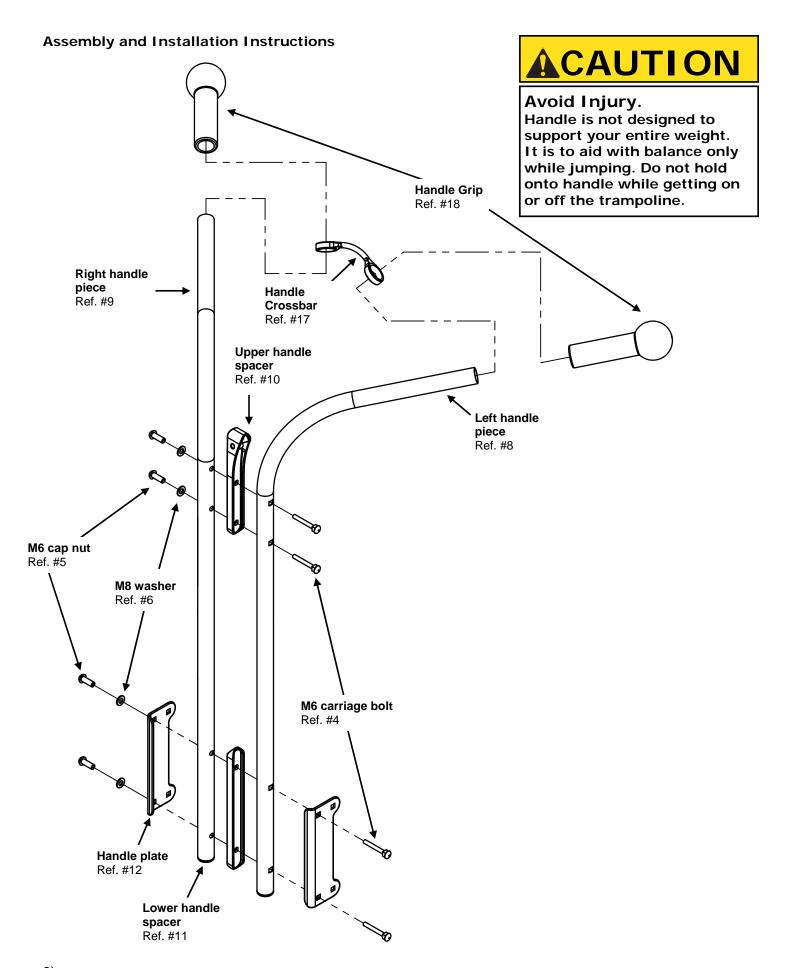
**2)** Assemble the handle, as shown, starting with the upper handle spacer. When completed, you will have a "handle assembly". *M6 bolts should only be hand-tight.* They will be securely tightened in a later step.
