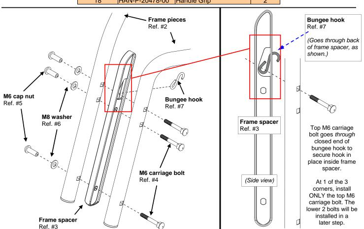
**1)** Assemble all 3 corners of the triangular frame. *M6 bolts should only be hand-tight*. They will be securely tightened in a later step.
