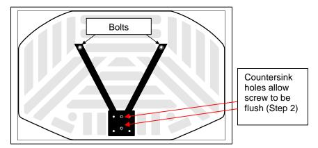
Step 2: Attach front plate with sides [B] to front of backboard.
