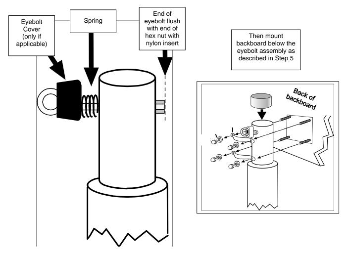
Install backboard assembly to the end of the pole as outlined in the instruction manual, and then hook the net into the eyebolt hook by pushing eyebolt cover toward pole. When net is in place, let the spring return the cover to close the hook.
