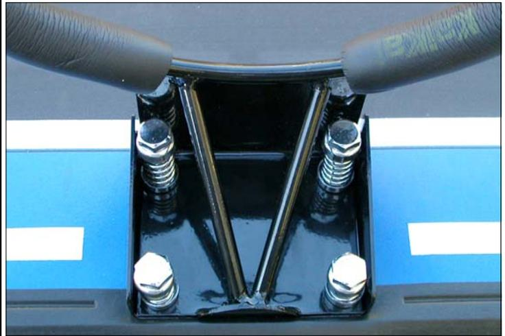
7) Insert the two M10 x 100mm bolts into top two holes of front plate and thread them through back plate and long brackets until long spring with thick wire will not slide along bolt. Then tighten bolt 1 full rotation and stop.
