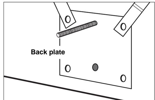
**3)** Insert an M8 screw through lower middle hole on back plate, and thread it through M8 standard nut on front plate. Tighten until screw is flush with nut on front of backboard, as shown. Do not over-tighten.
