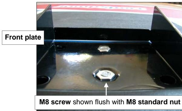
**3)** Insert M8 screws through middle holes in back plate, and thread them through M8 standard nuts on front plate. Tighten until screws are flush with nuts on front of backboard, as shown. Do not over-tighten.
