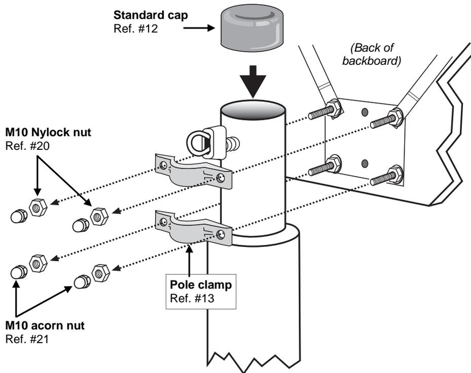
10) Install standard cap to top of pole. With the bolts straddling the enclosure pole (just below the eyebolt) install pole clamps and M10 Nylock nuts, as shown. Tighten all Nylock nuts evenly. Then *hand-tighten* acorn nuts on to end of M10 bolts.
