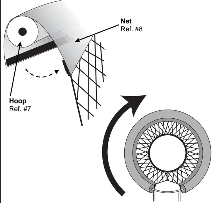
8) Detach Velcro connection around top of net. Place net over hoop. Reattach Velcro around hoop, working clockwise.
