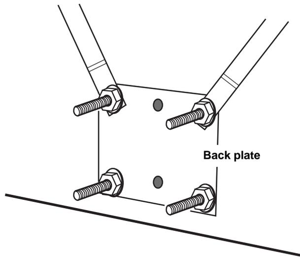
7) On back of backboard, place an M10 washer over all four M10 bolts sticking through back plate and long brackets. Then screw an M10 standard nut over each of the bolts. Thread the nuts down until they just touch the washers. Then tighten each nut 1 full rotation and stop.
