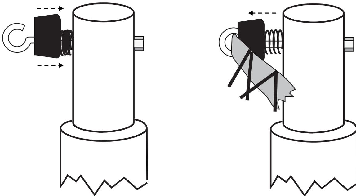
**11)** After backboard is mounted, push eyebolt cap toward pole, then place net into eyebolt hook. When net is in place, let the spring return the eyebolt cap to close the hook.
