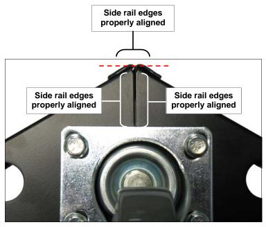
**6)** Make sure edges of side rails align properly, as shown. Then use a **1/2" wrench** (or similar) to snugly tighten down all 4 bolts.
