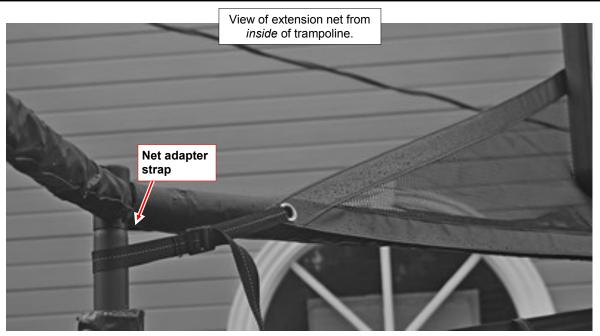
**6)** While standing on *inside* of enclosure net, stretch out end of one extension net toward closest safety enclosure pole. Wrap strap around enclosure pole above the enclosure pole pad. Be sure extension net is positioned on *inside* of enclosure net. Wrap strap through the grommet in the end of the extension net. Then secure end of strap through buckle and pull snugly. >> Repeat with extension net on opposite side.
