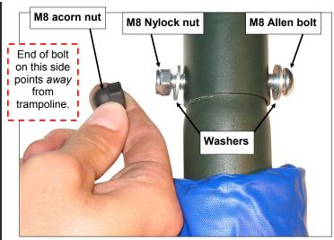
**5)** Using M8 Allen bolt, M8 Nylock nut, and M8 acorn nut (included with this kit), secure adapter pole with basketball set to top of safety enclosure pole. Tighten Nylock nut securely, but only hand-tighten acorn nut.
