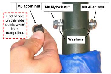
**3)** Using M8 Allen bolt, M8 Nylock nut, and M8 acorn nut (included with this kit), secure adapter pole with basketball set to top of safety enclosure pole. Tighten Nylock nut securely, but only hand-tighten acorn nut.
