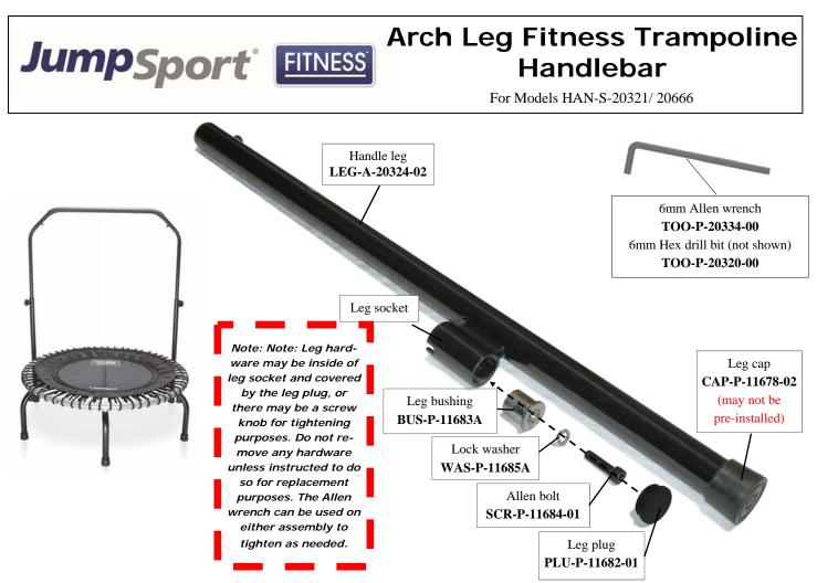
**1)** Familiarize yourself with the leg pieces (leg and leg cap) and the Allen wrench/drill bit. Leg hardware (leg bushing, lock washer, Allen bolt, and leg plug) may already be installed and covered by the leg plug.
