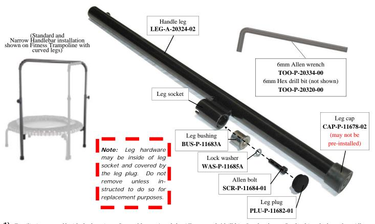
1) Familiarize yourself with the leg pieces (leg and leg cap) and the Allen wrench/drill bit. Leg hardware (leg bushing, lock washer, Allen bolt, and leg plug) may already be installed and covered by the leg plug.
