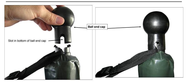
**4)** Connect ball end cap to top of pole. Slot in bottom of ball end cap will align with notch in top of pole. Ball end cap will lock into place when properly installed. Be sure short strap is not caught between ball end cap and top of pole. Do NOT tighten short strap. Leave short strap **loosely** connected for now.
