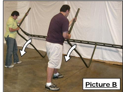
**9** Connect the nearby leg assemblies into the sockets on the bottom of the short rail piece, while the other person holds the rail assemblies steady (see Diagram 5).
